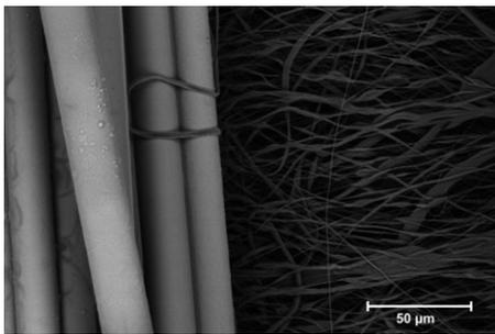
Fig. 3. SEM image of the interface between PCL nanofibers and bioactive glass microfibers in the double-layered bio composites.
