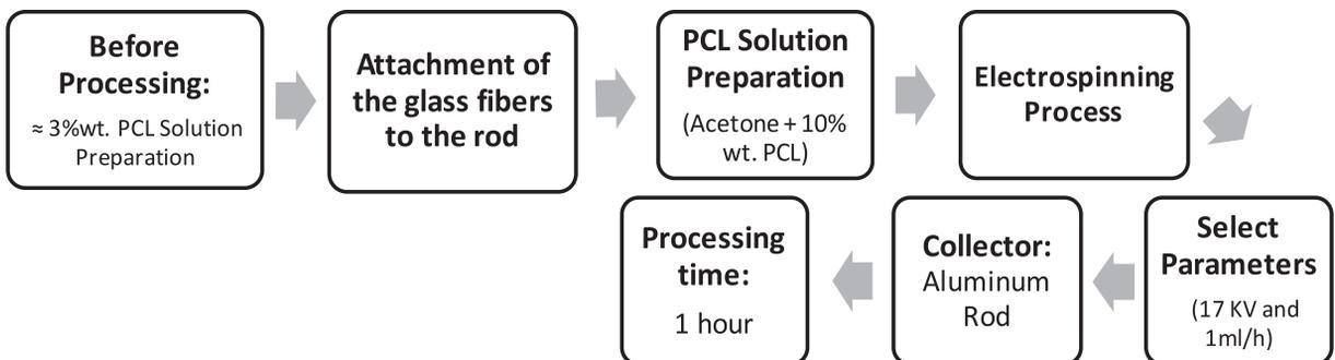
Fig. 1. Schematic diagram for the manufacture of the 2 types of composites: DL membranes and DL nerve guide conduits.
