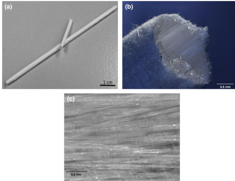
Fig. 2. (a) Double-layered nerve guides (DL) as prepared; (b) DL nerve guide with aligned fibers in its interior; and (c) aligned bioactive glass fibers in the interior of the nerve guide conduits.
