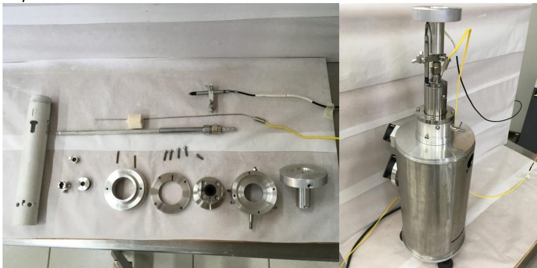
Figure I . Building steps of the new EDOS-HiV viscosimeter.
